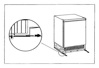
Removing covering and adjusting strips
